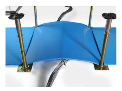
For under floor data cable routes, the Jezmat, data cable mat system is ideal. To complete the system a factory formed bridge arrangement is available. This quick, strong and versatile addition to the Jezmat range is specifically designed to fit between four pedestal legs within a 600mm x 600mm raised floor configuration. It allows the Jezmat route to cross other services including pipe work and track systems.
